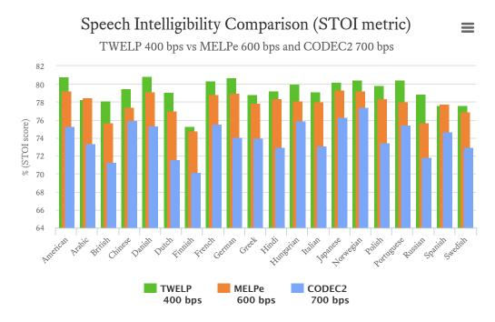
The diagram illustrates a difference in speech intelligibility between the TWELP 400 and MELPe 600 vocoders in the STOI metric. We've also included numbers for the free CODEC2 700 bps vocoder for comparison. Exact values are provided in the table below:
