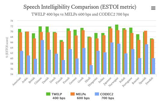
The diagram shows a difference in speech intelligibility between the TWELP 400 and MELPe 600 vocoders in the ESTOI metric. We've also included numbers for the free CODEC2 700 bps vocoder for comparison. Exact numbers are shown in the table below.
