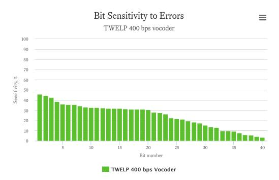
We strongly recommend using FEC (Forward Error Correction) with unequal protection of the bits in strong accordance with their sensitivity to errors and utilizing 'Soft Decisions' decoding. This will provide the highest robustness of the vocoder against errors in the channel.
