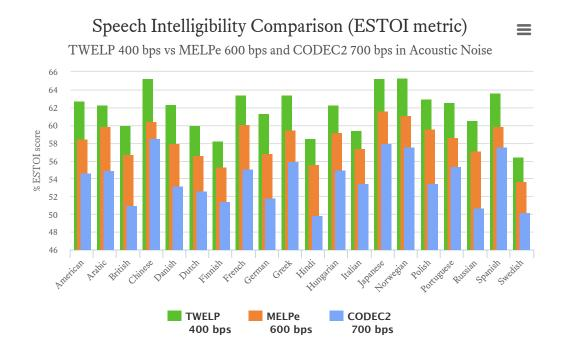
The diagram demonstrates a difference in speech intelligibility for noisy speech (SNR = 10 dB) between the TWELP 400 and MELPe 600 vocoders, based on the ESTOI metric. We've also included numbers for the free CODEC2 700 bps vocoder for comparison. Exact numbers are shown in the table below.
